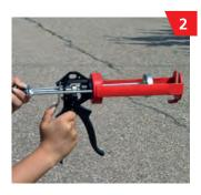
Clamp the cartridge into the appropriate dispenser\* for the cartridge size.
