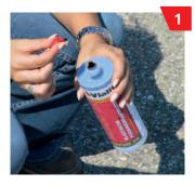
Open the cap of the cartridge and screw on the enclosed mixing nozzle\*.
