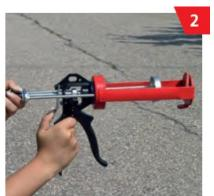
Clamp the cartridge into the appropriate dispenser for the cartridge size.
